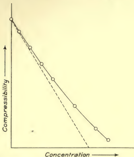
FIG. 17.—Compressibility of NaCl solutions in concentrations varying between 0 and 26.22 per cent. (According to H. Gilbaut.)
